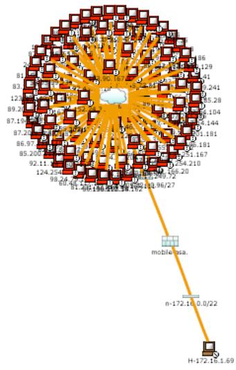
The host towards the bottom (172.16.1.69) is connected to a Bittorrent swarm on the Internet (the large circle of interconnected hosts towards the top of the image.)
