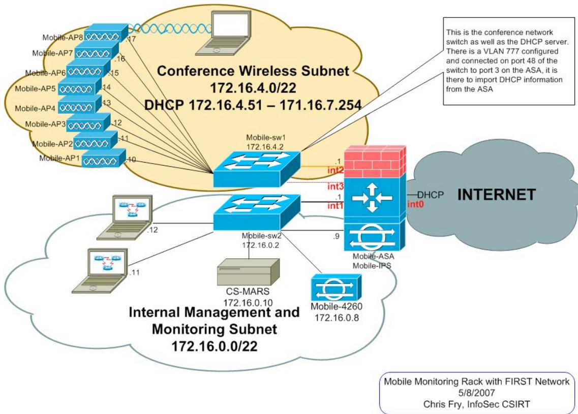
Here is the visualization created automatically by CS-MARS with all the security and network devices loaded:
