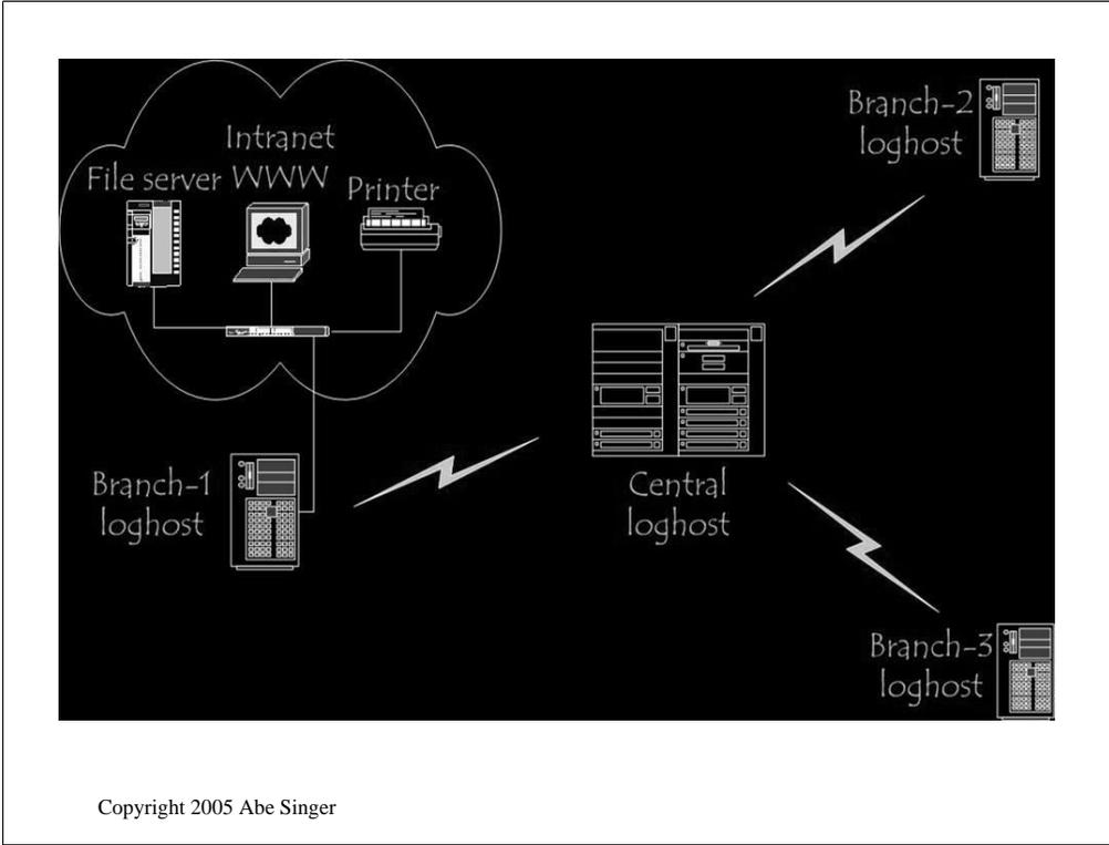
diagram of a relay architecture
