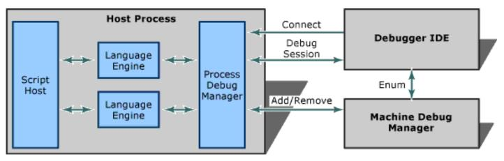
Machine Debug Manager (mdm.exe) and Process Debug Manager (pdm.exe) are part of the Microsoft Script Debugger. Implementing the required interfaces of the Debugger IDE (IApplicationDebugger) allows one to set breakpoints and inspect variables in real-time.
