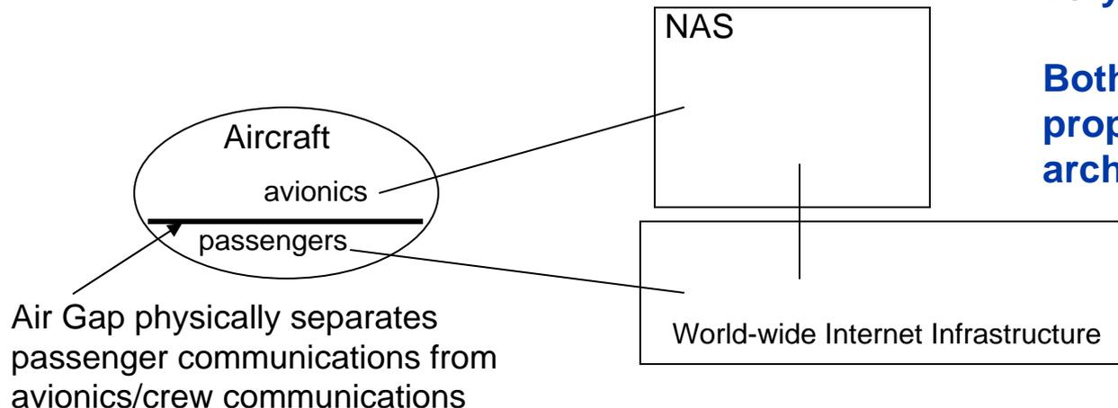
Air Gap physically separates passenger communications from avionics/crew communications
