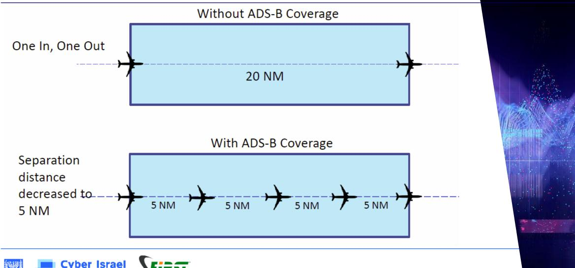
**ADS-B Out** is the broadcast part of ADS-B. An aircraft equipped with ADS-B Out capability will continuously transmit aircraft data such as airspeed, altitude, and location to ADS-B ground stations.
